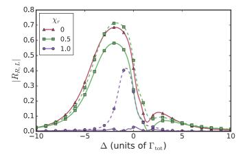
FIG. 10. Reflection spectra for weak-scattering configurations, calculated via transfer matrix. Dashed lines represent  $|R_L|$ , the reflected amplitude of left-propagating light, while solid lines represent  $|R_R|$ .
