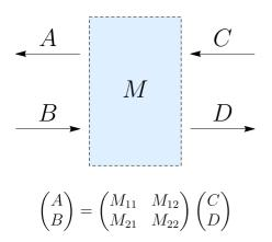
FIG. 8. Illustration of how the transfer matrix can be used to calculate the fields on one side of an optical element given fields on the other side.
