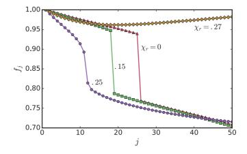
FIG. 5. Evolution of the phase-slip configurations as  $\chi_r$  increases from 0 to 0.27 at  $\delta = \Gamma_{\text{tot}}$ . These are produced by the numerical protocol outlined in Sec. II B.
