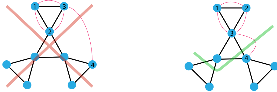
Figure 3.11: An illustration of how and why the process of rotation works in our circuit placement algorithm. In this diagram, red links represent gates to be performed (edges in C ) and black ones are available communicative links (edges in M ). In the graph C , the qubits 1, 2, and 3 are all connected, and 3 is connected with 4. These qubits have been correctly placed into clusters (1, 2, 3) and (4). However, if they are not rotated correctly (see left), the link between 3 and 4 can become quite long, necessitating a long-range quantum gate. By properly rotating (right), the gate between links 3 and 4 becomes much shorter, improving the placement.
