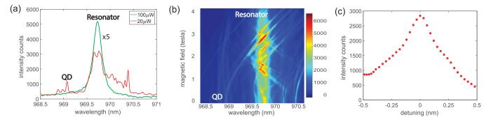
FIG. 5. Purcell enhancement of a quantum emitter coupled to a topological resonator. (a) The measured PL, at zero magnetic field, exhibiting the QD and the resonator mode at high and low excitation power. (b) Enhancement of emitter's PL, when the QD is tuned to the topological resonator, by scanning the magnetic field. (c) The intensity of the QD's emission, as a function of detuning from the resonator mode.
