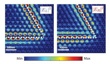
FIG. 6. Simulated left/right circular polarization components of the electric field. The white dotted line marks the perimeter of the resonator.
