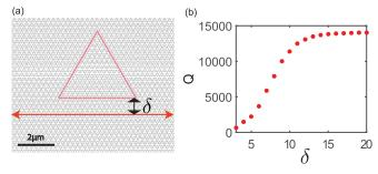
FIG. 8. (a) Schematic of the simulation setup. Red super-triangle indicates the resonator perimeter. The double-arrowed red line indicates the position of the waveguide. (b) The quality factor (Q) versus distance ( $\delta$ ), showing saturation of Q at high values of  $\delta$ .
