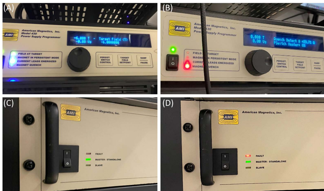
Figure E.5: (A) The magnet controller operating correctly at a target field of -6T. (B) The magnet controller reporting a quench event that must be reset. (C) Magnet power supply operating correctly. (D) Magnet power supply experiencing a fault event.
