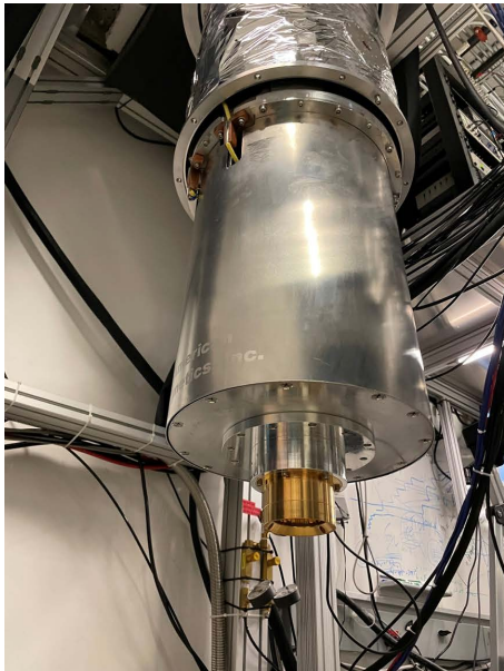
Figure E.1: Image of the magnet attached to the 4k middle radiation shield. Spec sheet supplied by American Magnetics. The most important value is the Field to Current Ratio which must be entered into the controller unit to calibrate the field values.
