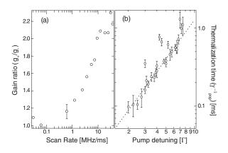
FIG. 4. (a) The ratio of peak gain  $(g_-/g_+)$  indicates a limiting scan rate  $d\delta/dt \approx 0.5$  MHz/ms below which decoherence and thermalization of the momentum distribution suppress optical bistability. The data were obtained at a pump detuning  $\Delta \sim -4\Gamma$ . (b) Thermalization time  $(\gamma_{pop}^{-1})$  vs the pump detuning. A fit to the data (dashed line) indicates a power-law dependence  $\gamma_{pop}^{-1} \propto \Delta^{\alpha}$  with  $\alpha = 1.57 \pm 0.09$ .
