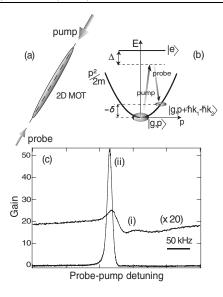
FIG. 1. (a) Schematic indicating the pump and probe beams used for the RIR, where MOT is the magneto-optic trap. (b) The energy levels relevant to the RIR. (c) Absorption spectrum of a probe beam around the RIR for longitudinal optical depth of  $\sim 10$  (i) and  $\sim 40$  (ii).
