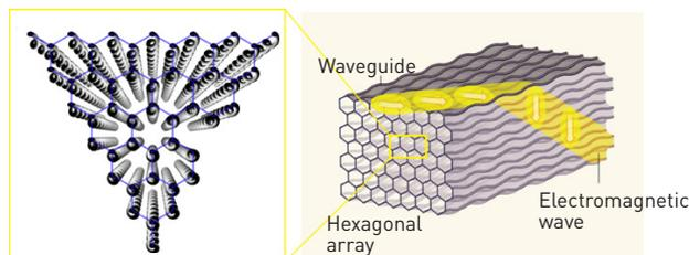
A 2-D lattice of helical waveguides in which z-symmetry is broken simulates, in space, the breaking of time-reversal symmetry characteristic of Floquet topological insulators.
